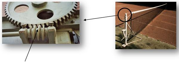
A worm and gear wheel are used to tighten tennis nets. A small force used to turn the crank handle produces a large force to stretch the net.
