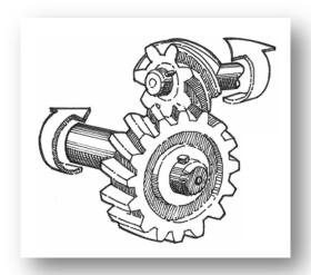
When considering the speed changes in most worm gear systems, you can think of the worm as if it were a spur gear with one tooth. It is a single tooth wrapped around a cylinder. 1 turn of worm gives a rotation of only one tooth by the driven worm wheel. (Note that worm gears can only be used to REDUCE speeds and not increase speeds. If you try and rotate the driven gear it will jam against the worm).
